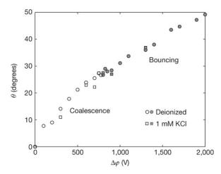
The contact angle  $\theta$  of the double cone for water droplets in air with applied potential  $\bigtriangleup \varphi$ . Open symbols denote coalescence, filled symbols denote bouncing. Reprinted by permission from Macmillan Publishers Ltd: Nature, WD Ristenpart et al. **461**, 377-380, ©2009, doi:10.1038/nature08294.
