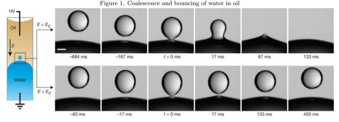
A high-voltage (HV) provides the electric field of strength E. The top row of images shows coalescence ( $E < E_C$ ) whereas the bottom row shows bouncing ( $E > E_C$ ) of the water droplet. Reprinted by permission from Macmillan Publishers Ltd: Nature, WD Ristenpart et al. **461**, 377-380, ©2009, doi:10.1038/nature08294.
